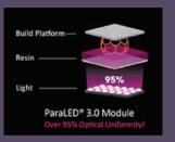
Unlike conventional COB LED design, Phrozen uses ParaLED 3.0 Module (parallel UV LED matrix back light system) giving the Sonic XL 4K the ability pass light through resin with complete uniformity.
